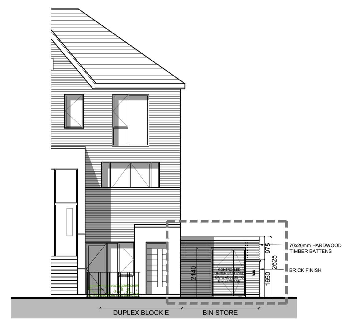
BIN/BICYCLE STORE NO. 3 - SIDE (SOUTH) ELEVATION Scale 1:100
