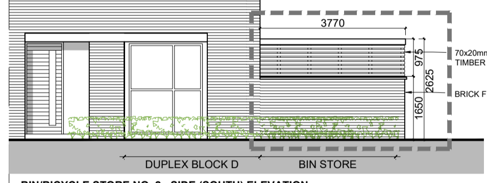
BIN/BICYCLE STORE NO. 2 - SIDE (SOUTH) ELEVATION Scale 1:100
